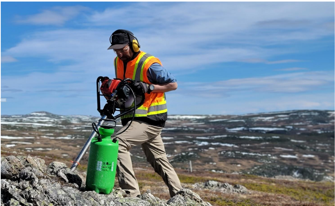
Figure 3: Hand-held Power-Auger Sampling Outcrop
