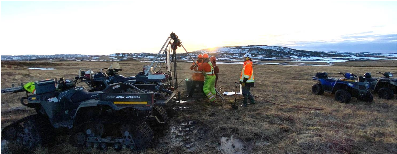
Figure 2: ATV-mounted Power-Auger drill at Window Glass Hill
