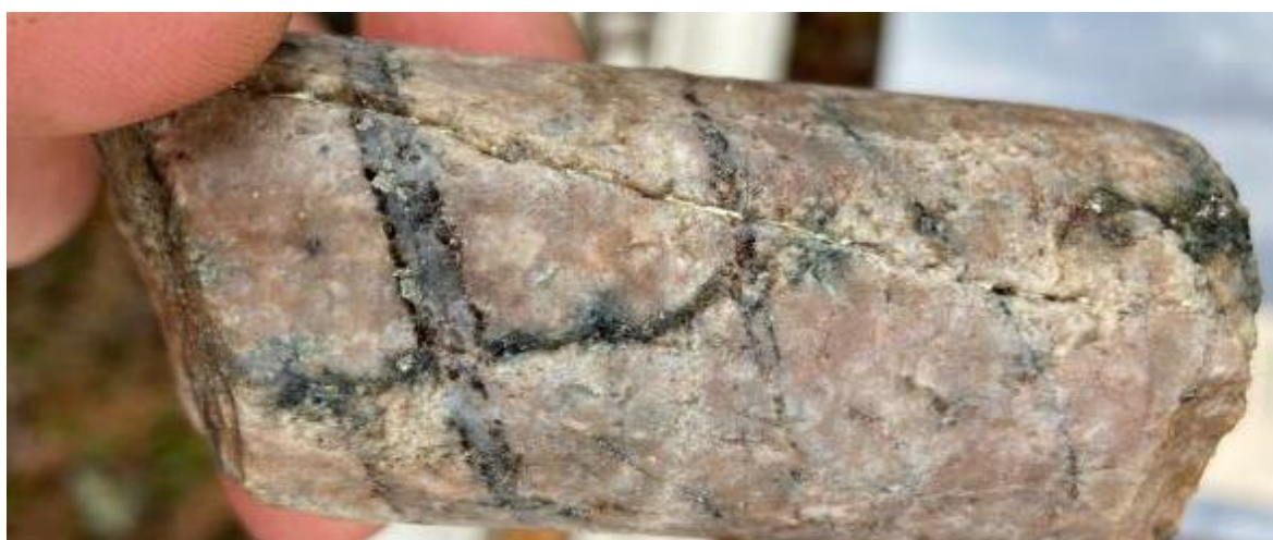
Figure 1: Bottom of hole core from Power-Auger drill hole 5717 showing typical WGH-style vein assemblages - from a previously untested area of the Window Glass Hill Granite
